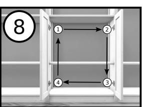
If adjusting 2 or more doors together ensure all adjusting screws are set to the same position before starting.
