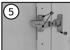
Fix the backplate to the upright using the self tapping screws at the centre of the slots, it should be aligned almost flush with the back of the upright.
